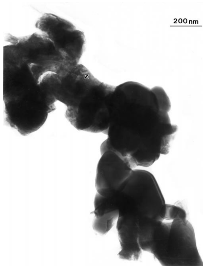
FIG. 7. Low-magnification micrograph of pure Series B \text{Nd}_2\text{O}_3 . The grain marked z is an example of the platelike material occasionally seen in this sample.
