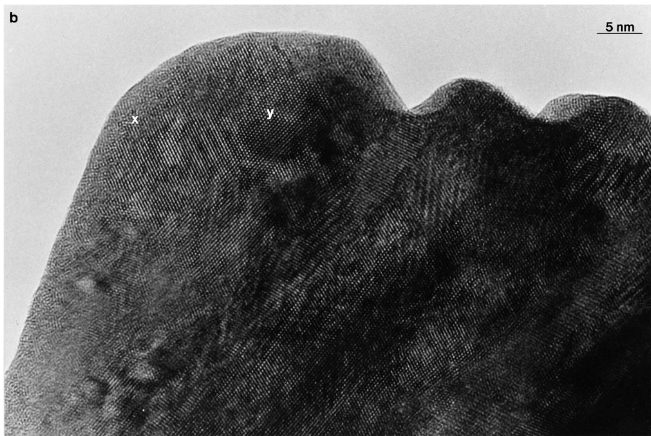
FIG. 1. (a) Low-magnification image of Series A undoped \text{Nd}_2\text{O}_3 . (b) The complex microstructure at higher magnifications: x, disordered/semi-crystalline material; y, highly ordered crystalline material.
